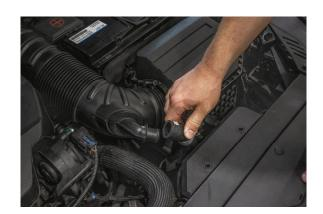
5 Disconnect the 2 rear re-circulation pipes from the rear of the intake
