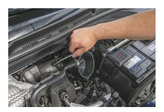
12 Identify the rubber blow-off hose required. The shorter hose is for pre-face lift cars and the longer one for post-facelift cars.
