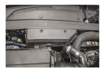
8 Lift out the airbox and intake pipe.
