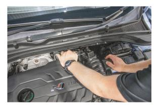
6 Undo the 3 M6 screws using a 10mm socket securing the airbox base.
