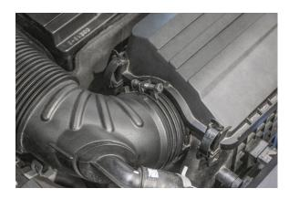
3 Loosen the hose clamp that connects the OE hose to the turbo inlet
