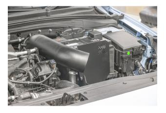
$20 \qquad \text{Connect the two breather hoses to the top of the intake pipe using } \\ \text{OE spring clamps}.$
