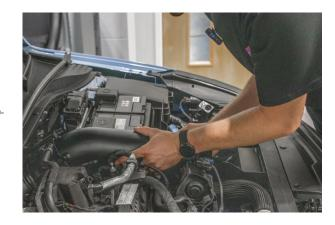
$18 \qquad \text{Align the pipe bracket with mounting stud hole and reinstall the } \\ \text{mounting stud.}$
