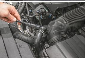
$2\,$   $\,$  Loosen the hose clamp that connects the OE hose to the airbox
