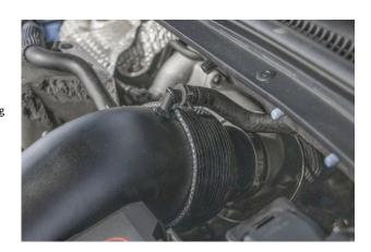
21 Install the 20° silicone joiner with a jubilee clamp to the front of the intake pipe.
