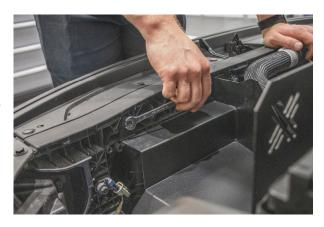
$17 \qquad \text{Install the intake pipe in to the silicone reducer, use one of the 100-} \\ 120 \text{mm jubilee clamps, don't tighten yet.}$
