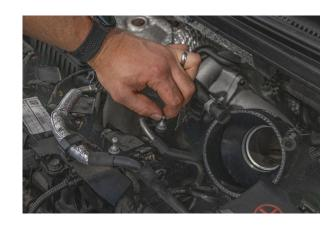
$14 \quad \text{Place the heatshield in to the engine bay, locating the heatshield} \\ \quad \text{bracket on to the already fitted anti-vibration mount.}$
