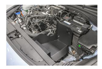
Secure the heatshield using the supplied M6 nyloc nut on the anti-vibration mount.
