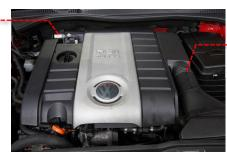
3 Remove the turbo inlet pipe using circlip clamps or pliers.
