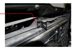
7 Loosely install heathsield bracket B onto the heatshield in the position shown using an M6 bolt, 2 x M6 washers and M6 nylock.
