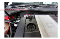
Unclip the two silver clips next to the MAF holding the intake pipe to the airbox. Next using circlip clamps or pliers remove the front intake duct from the airbox. Pull up on the airbox assembly and remove.
