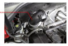
4 Remove the front air duct by removing the two self-tap screws holding it in place.
