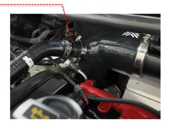
10 Remove the MAF unit from the stock airbox using a T20 torx bit. Next install the MAF unit into the new Intake pipe using the supplied M4 bolts and washers in the pipe as shown and secure using a 3mm Allen key.
