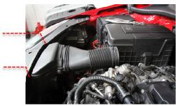
Install the new silicone elbow onto the turbo using the OE tension clamp from the old intake pipe.
