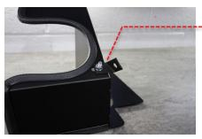
8 Install the heatshield as shown, fix into position by using an M6 bolt and M6 washer to bolt bracket B to the mounting post next to the battery tray. Next using an M6 bolt, 2 x M6 washers and M6 Nylock secure the front of the heatshield to bracket A you installed earlier. Once all bolts are in place go around and ensure they are all tightened and secure.
